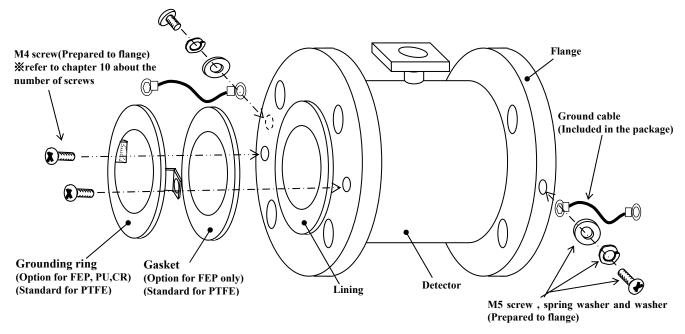
Figure 4.4 Install of grounding rings and ground cables
